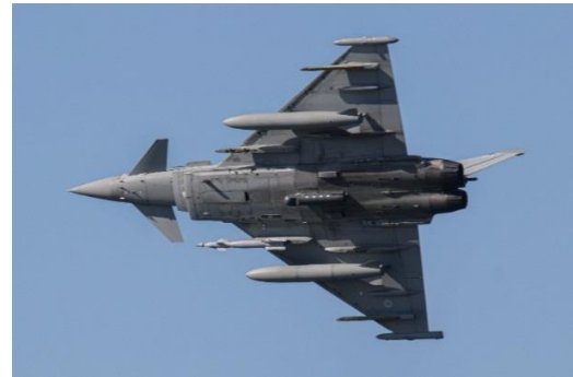
A Typhoon loaded with a single Paveway IV Laser-Guided Bomb a Laser Designator Pod overflying the tower at Garvie.
